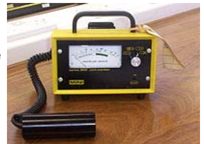
A Geiger counter, that detects and counts radio active emissions. Different tubes are used for \alpha , \beta & \gamma radiation
