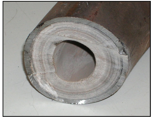
Above. This is a section of a copper water pipe on the outer wall over many years lime scale has been deposited the point where the amount of water the pipe can carry is very much reduced. Doncaster's water is borehole sourced, and as a consequence is a known source of hard water. This is a problem is known as the 'Cholesterol of Plumbing'.
