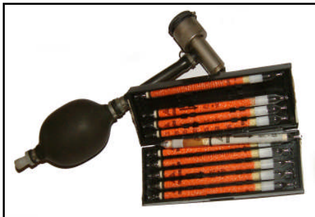
It was not until the 1960s-70s that portable testing equipment became available. These comprised of Dragger tubes, where the air sample was pumped through glass by a rubber bulb. The tubes contained a chemical which changed colour in the presence of Carbon monoxide and other dangerous gases. Since then, more modern electronic equipment has become available.
